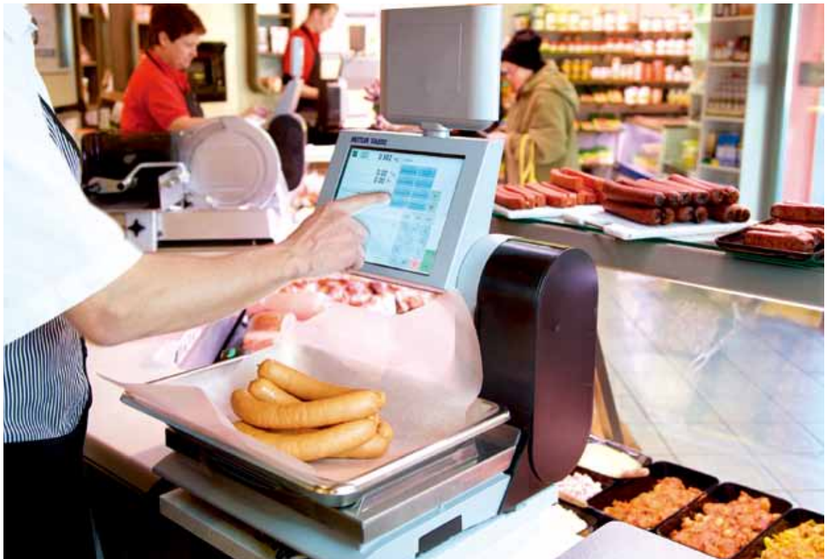
For Hanspeter Fischli, a key advantage over classic keypads is that the smooth touchscreen interface is easy to clean and has no edges or ridges where dirt can collect. "Even the cable connections have been cleverly designed to maintain a hygienic workplace", explains Hanspeter Fischli.
