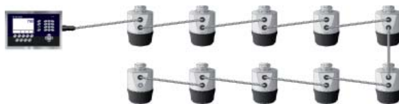
A cell-to-cell network, designed to eliminate junction boxes and limit the number of connection points
