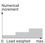
• MultiInterval precision means automatic switchover of the numerical increment (readability) in dependence on the applied load.
